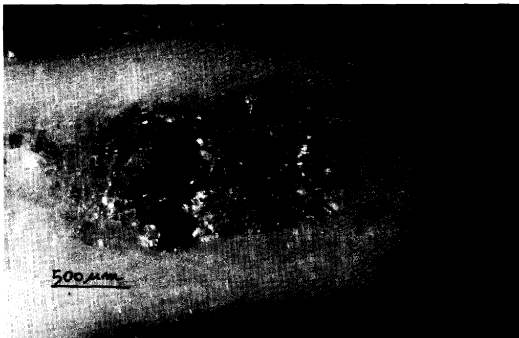
Fig. 3. Cross-section of partially crystallized sample. Glass melted in Pt crucible.
